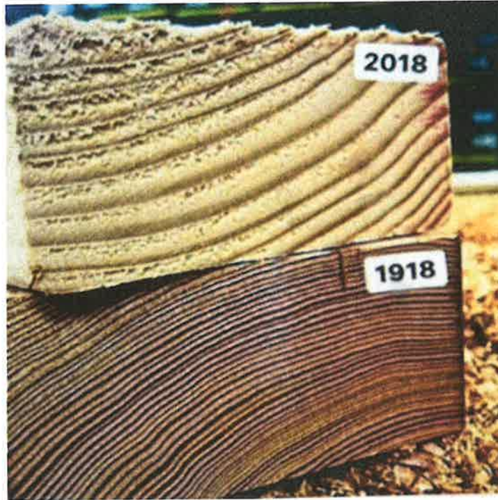
Photo from Secretary of Interior Preservation Brief 16 showing how new wood is much less dense than old growth lumber.
